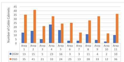
Fig. 8: The number of cable cabinets from the OGM and DSO datasets based on an eight-meter distance threshold.
