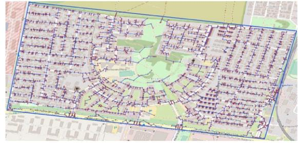
Fig. 13: The DSO-inferred model of the Freimann subarea.
