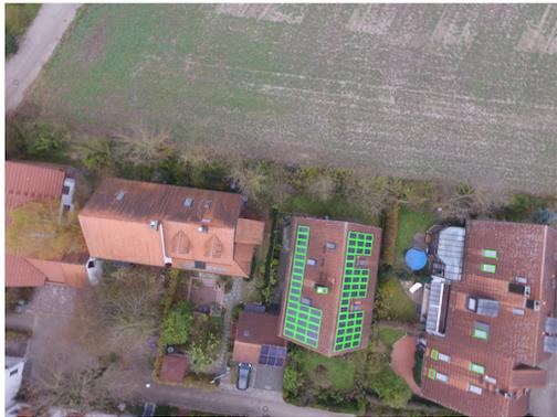
Fig. 18: The result of nonmaximum suppression (in green) combining the detected contours.
