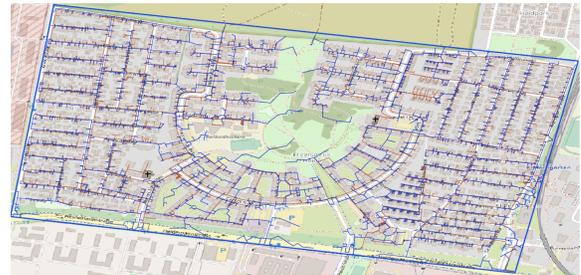
Fig. 15: Overlapping ground-truth and DSO inferred-models. (Orange lines are ground truth, and the blue lines are DSO.)
