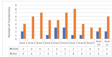
Fig. 9: The number of transformers from the OGM and DSO datasets based on an eight-meter distance threshold.
