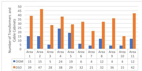
Fig. 7: The number of transformers and cable cabinets from the OGM and DSO datasets based on an eight-meter distance threshold.
