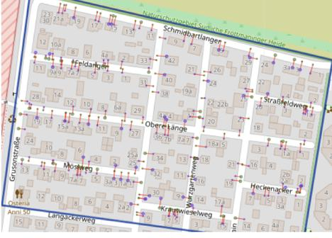
Fig. 10: Projection of the target node on the nearest roads with an edge between them.
