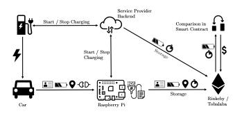
Figure 1. The workflow of a charging event.
